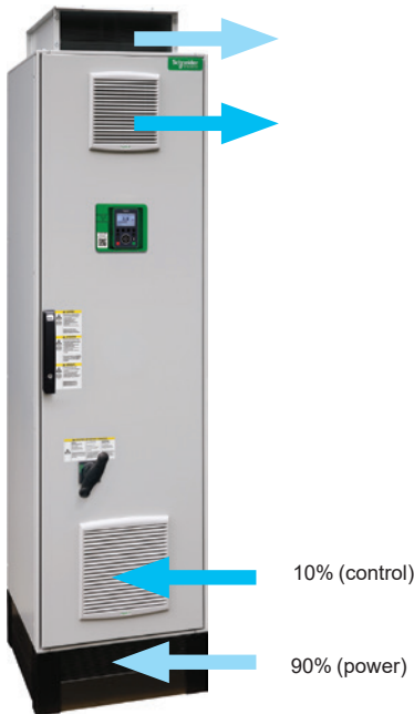
Cooling system with two separate air flows
